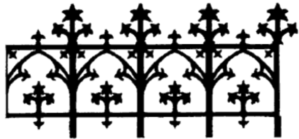
Cast Iron Roof Cresting
